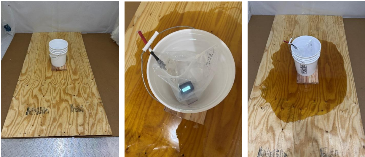
Figure 8: Chemical Spill Simulation prior to and after spill
