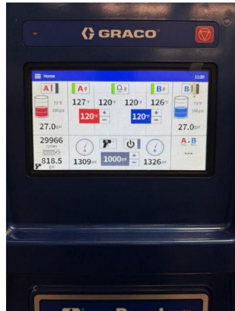
Figure 6: Proportioner Screen showing 22.0 gallons of EnviroSeal OC Platinum used
